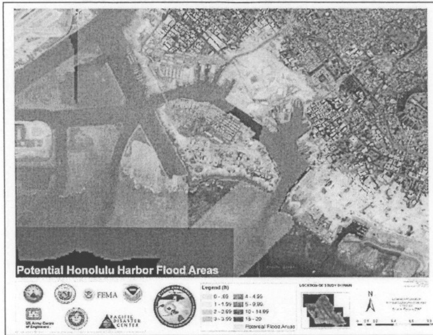
Figure 2.-6: Flood awareness areas, and areas of inundation on Sand Island due to seawall overtopping.
